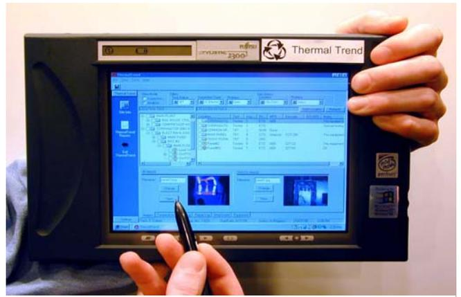
By using a pen computer running the database in the field, this allows the thermographer to enter problem information quickly into the database at the time of the inspection. This eliminates the need for typing up the report at the office.
