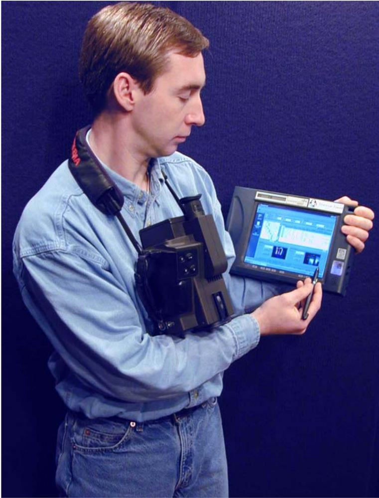
Thermographer with camera and Mobile Pen Computer running the Thermal Trend Infrared PdM Inspection Management Database.
